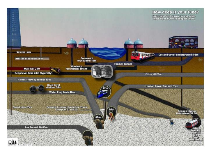
A section through the ground to indicate the depths which tunnels and services reach. This also shows how many tunnels there are and how deep they are in relation to the Thames.
