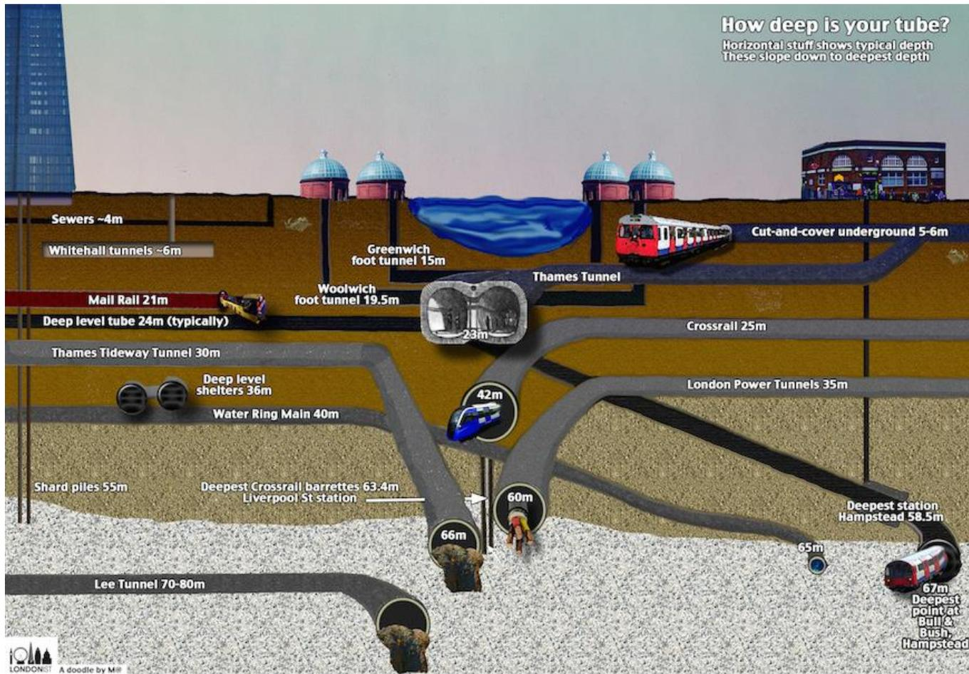
A section through the ground to indicate the depths which tunnels and services reach. This also shows how many tunnels there are and how deep they are in relation to the Thames.
